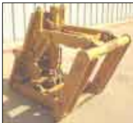
140M LIFT GROUP 293-5556
